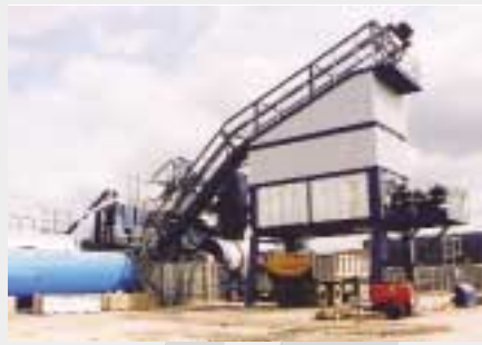
Free standing 120 tonne mixed material storage
