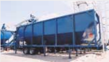
Mobile horizontal filler storage silo
